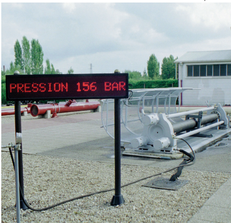
Destructive pressure test on a DN 250 pipe
