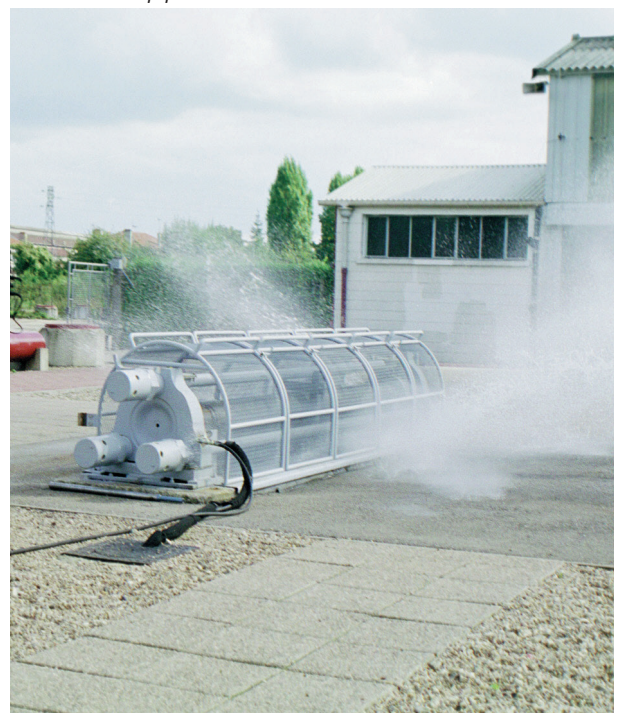
Destructive pressure test on a DN 250 pipe
