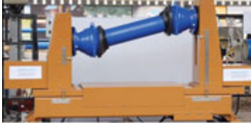
Deflection capability, thanks to the 2 ball flanges, capable to absorbing up to +/- 38°.
