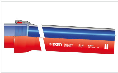
Ensemble Tuyau Standard INTEGRAL Ductan + Joint Standard
