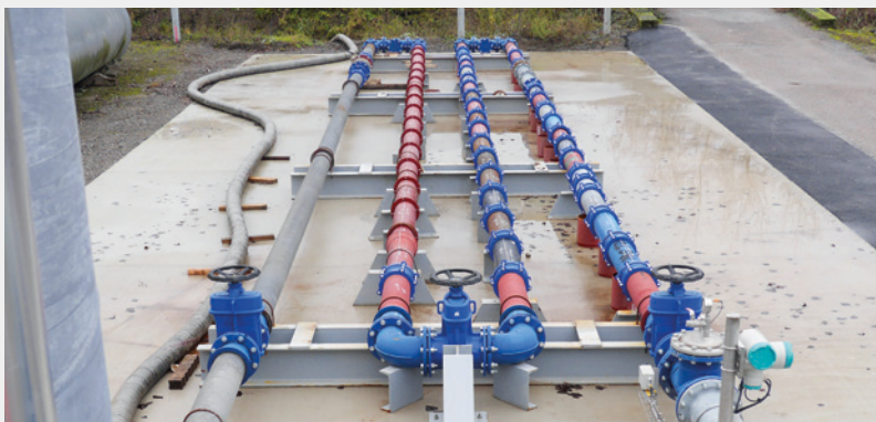
Abrasion loop at the Technocentre of PAM, in Mairières (Meurthe-et-Moselle, France): tests on the DUCTAN® internal coating.
