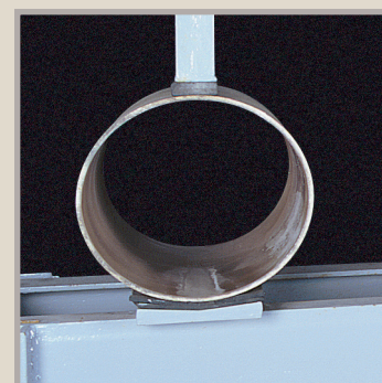
Crushing strength of a GRP tube
