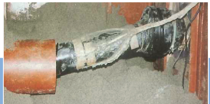
Test bed designed to recreate seismic earth movements: GEOFLEX® DN 150 - Deflection 200m
