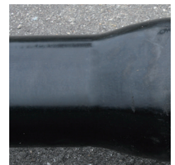
Appearance of the TT-PE coating for DN ≤ 500
