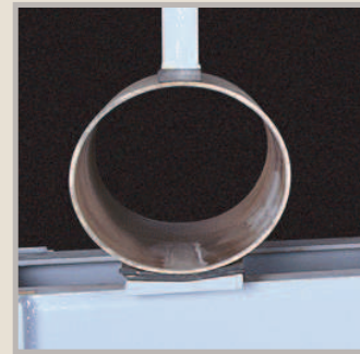
Crushing strength of a GRP tube
