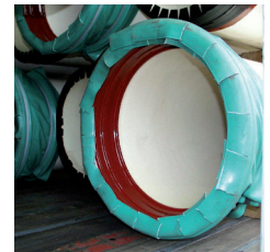
Protection of TT PUX pipes for transport
