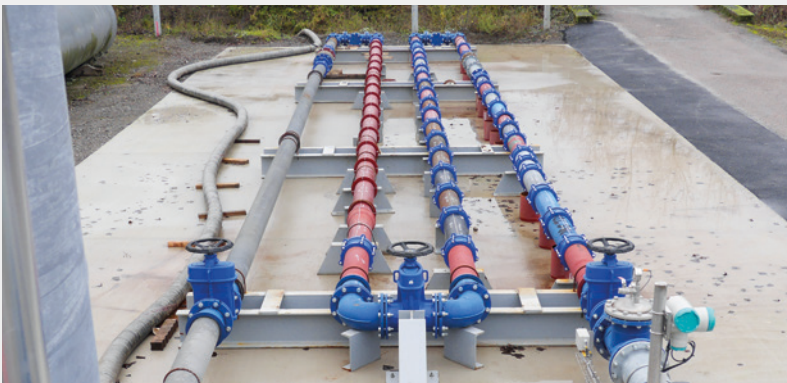
Abrasion loop at the Technocentre of PAM, in Mairières (Meurthe-et-Moselle, France): tests on the DUCTAN® internal coating.
