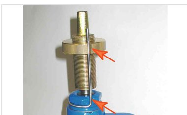
7- Stem places from there in the notch of the bearing nut and the index
